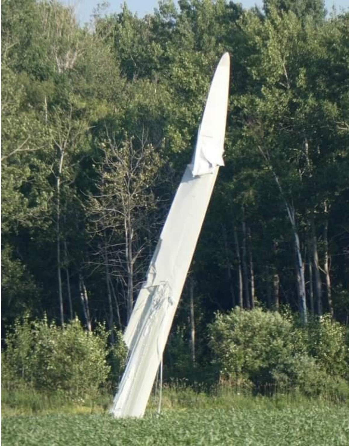
**Blade portion of failure at Capstone Skyway 8, June 30, 2021. Major portion of the blade was injected into the ground, at speed. Roads were closed for safety.**
